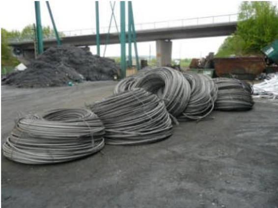
Image 55: aluminium wire with steel inliner
