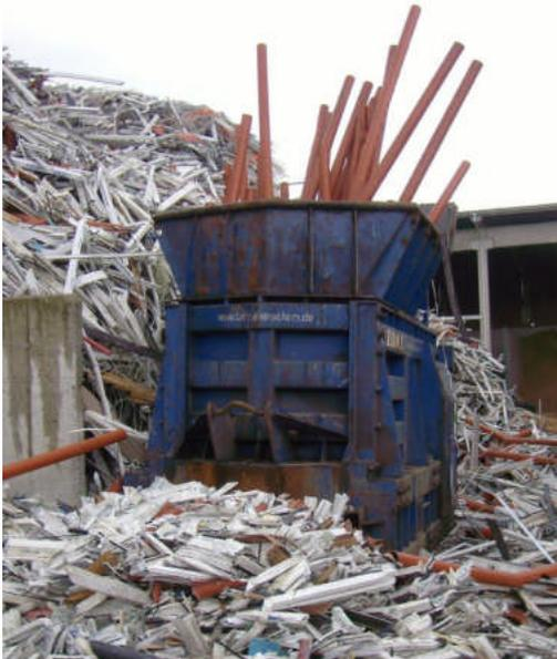
Image 65: PVC-piping in shear
