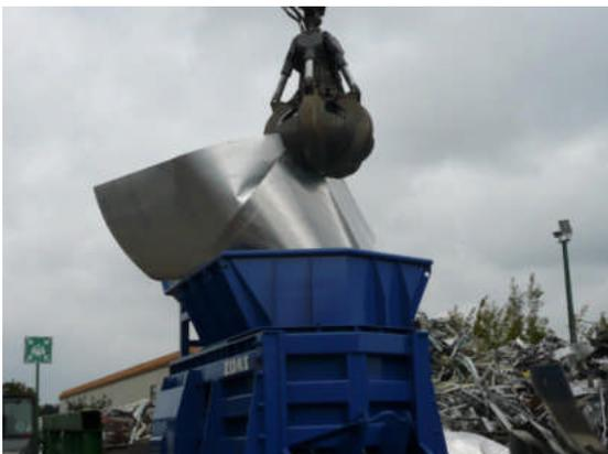
Image 38: Aluminium sheets in feed hopper
