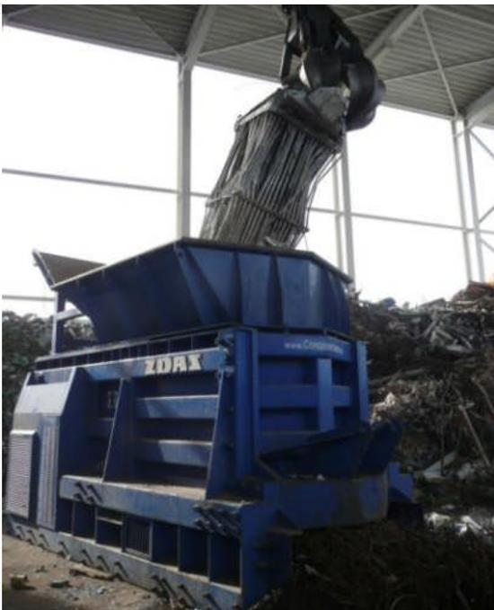
Image 25: heat exchanger in feed hopper
