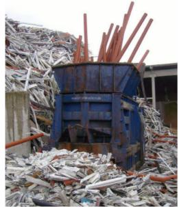
Image 65: PVC-piping in shear
