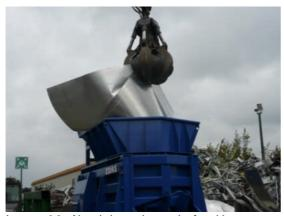
Image 38: Aluminium sheets in feed hopper
