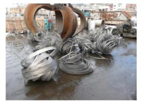
Image 48: Coil excess/trimmings
