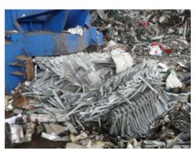
Image 26: Cut heat exchanger
