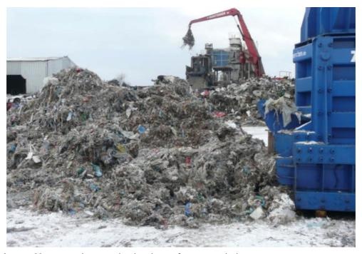
Image 68: cut steel paper plastic mixture from paper industry
