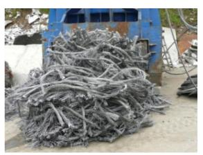
Image 56: cut wires with steel inliners
