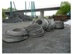
Image 55: aluminium wire with steel inliner
