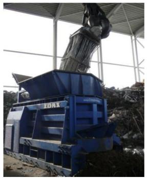
Image 25: heat exchanger in feed hopper
